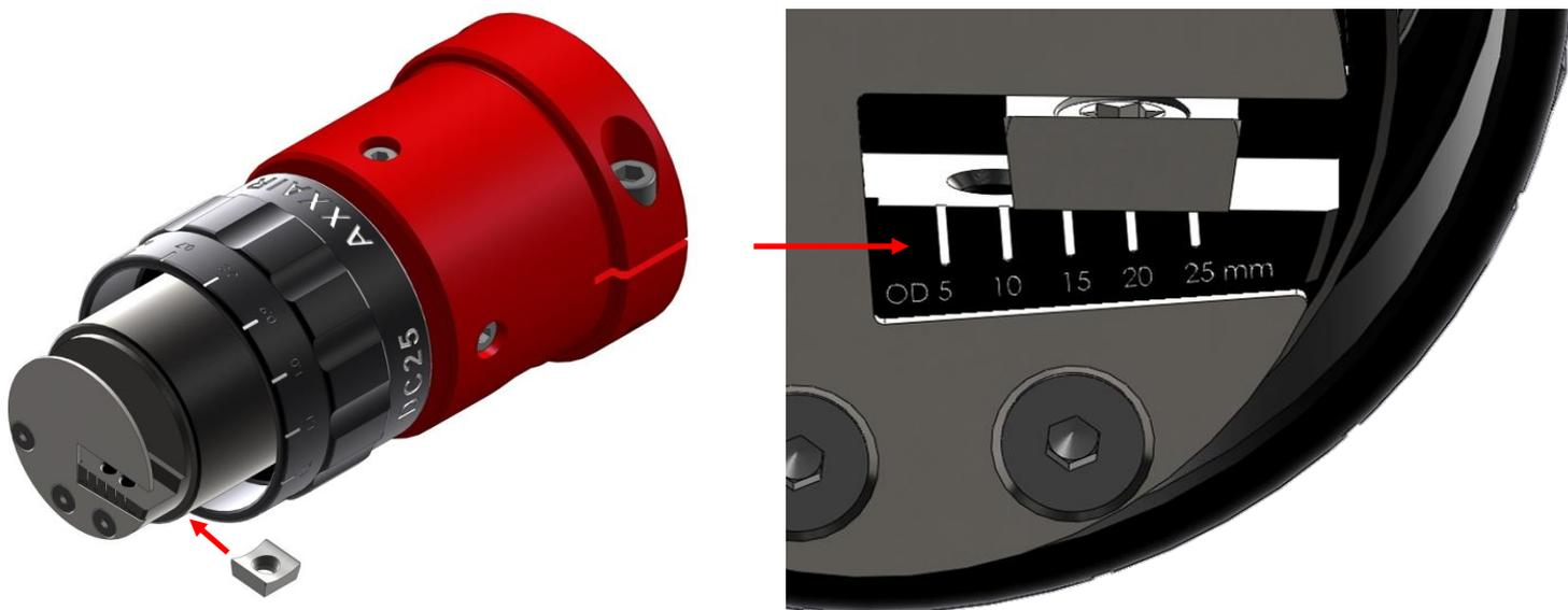
Then put in place and tighten the plate screw (tightening torque = 2.55 Nm, Torx T15 screwdriver supplied).
